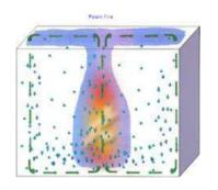
Steam pressure prevents oxygen feeding the fire – cooling hot combustion gases
